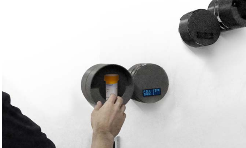
Fig. 1.1 Photo collage illustrating a SORT prototype delivering a medication bottle to user at scheduled time with prompt reminder.
