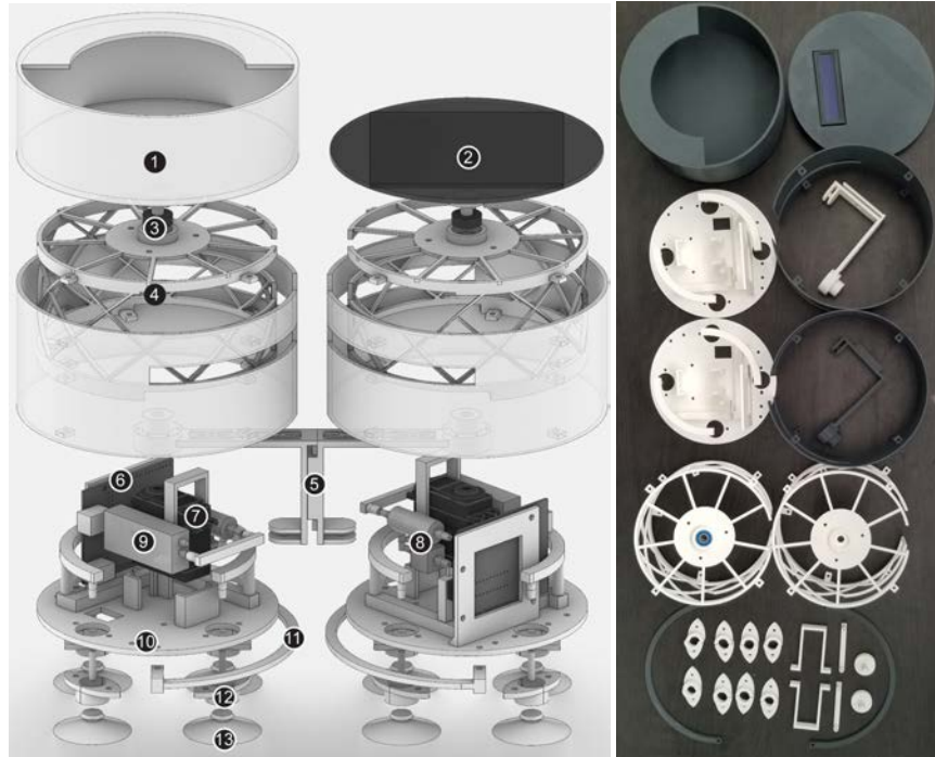
Fig. 1.9. Left: exploded isometric showing the robot components: 1) Receptacle container, 2) Display, 3) Magnetic connector with ball bearing, 4) Interior frame, 5) Connector bridge, 6) Micro-controller, 7) High torque servo, 8) Check valve + release valve, 9) Micro vacuum pump, 10) Base with integrated channels, 11) Bridge rails, 12) Suction cup anchor, 13) Suction cup. Right: 3D printed parts for constructing the prototype.
